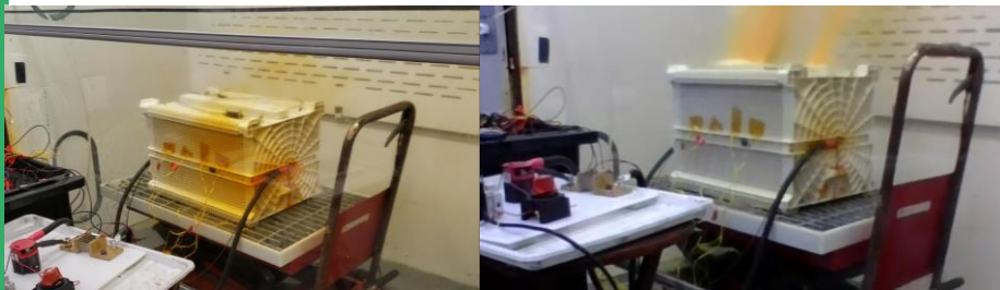
Some venting of steam, over 425A current (>20x nom.) on a 20A rated battery.
