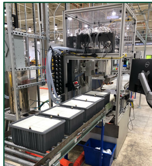
Z3 batteries at fill station
